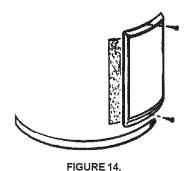
Remove the insulation cap with handle to expose the terminal cover.
